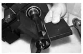
Place the machine in the bore. Hold to good start height, and tighten hand nut to snug. Push down on hand nut. While holding nut down, turn rod handle to tighten chuck.
